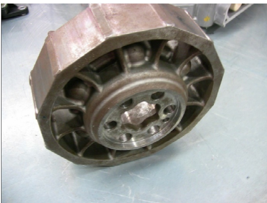
Figure 5 / The core or rotor is made of very strong rare earth metal permanent magnets
